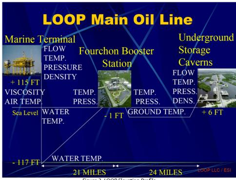
Figure 2. LOOP Elevation Profile
