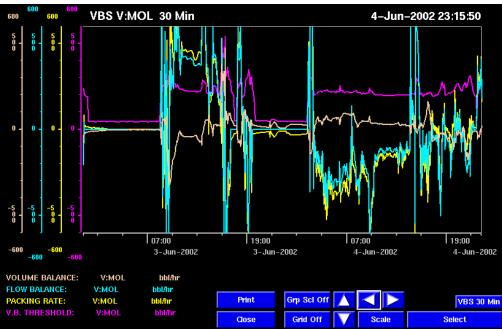
Figure 7. Leak Detection Trend, Tracking is Good with No False Alarms
