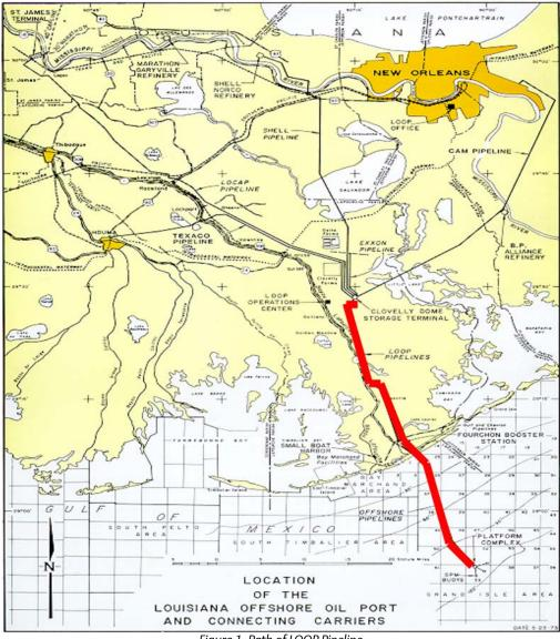
Figure 1. Path of LOOP Pipeline
