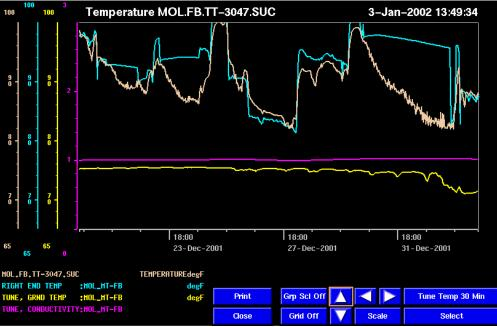
Figure 11. Trend with Measured and Calculated Temperatures during Numerous Shutdowns
