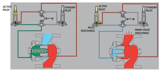
TYPE 63EGLP AT NORMAL CONDITION (BOTH MAIN VALVE AND ACTIVE PILOT ARE CLOSED)
