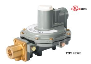
Type R632E has 1/8 in. NPT built-in gauge taps orificed to a No. 54 drill size, on the upstream and downstream sides. These taps provide easy access for testing the proper operation pressure of the First and Second-Stage while the system is pressurized. This regulator also features a large 3/4 in. drip-lip vent to reduce the chance of blockage by freezing rain or sleet when properly installed with the vent pointing down.
