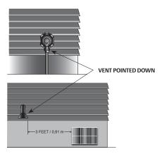
VENT INSTALLATION AWAY FROM WINDOWS, BASEMENT AIR INTAKES AND OTHER OPENINGS
