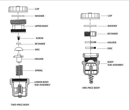
**EXPLODED VIEW OF TYPICAL FILLER VALVE CONSTRUCTIONS**
