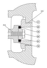
O-RING SEAT DETAIL FOR TYPE 99 REGULATOR WITH TYPE 61L (LOW PRESSURE) OR 61H (HIGH PRESSURE)
