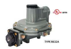
Type R632A has 1/8 in. NPT built-in gauge taps orificed to a No. 54 drill size, on the upstream and downstream sides. These taps provide easy access for testing the proper operation of the First and Second-Stage while the system is pressurized. This regulator also features a large 3/4 in. drip-lip vent to reduce the chance of blockage by freezing rain or sleet when properly installed with the vent pointing down.
