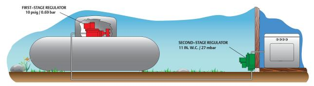
**Figure 1.** Two-Stage Regulation, One at Tank and One at Building, Reduce Pressure Down to Burner Pressure (11 in. w.c. / 27 mbar)
