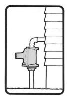
Second stage regulators should always be installed with the vent pointing down. This reduces the possibility of freezing rain or sleet plugging the vent. It also makes it more difficult for foreign material (pipe scale, dirt) to enter the regulator.
