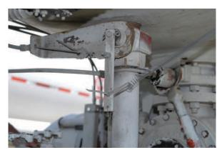
TO OBTAIN FULL OPERATING LEVER TRAVEL WITH SOME CABLE CONTROLS, THE CABLE HAS TO BE ATTACHED CLOSE TO THE HANDLE PIVOT
