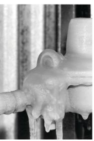
VENTS ON HORIZONTALLY MOUNTED REGULATORS BECAME QUICKLY PLUGGED DURING FISHER'S TESTS.
