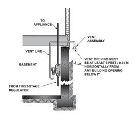
TYPICAL INDOOR INSTALLATION WITH VENT LINE AND VENT ASSEMBLY
