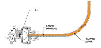
The figure above shows the condensate turned to ice at the orifice. This causes a freeze up unless the action of the regulator can break the ice jam.
