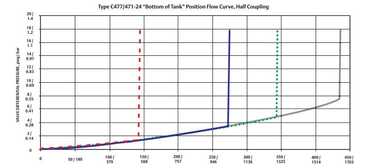
FLOW RATE, GPM / I/min PROPANE
