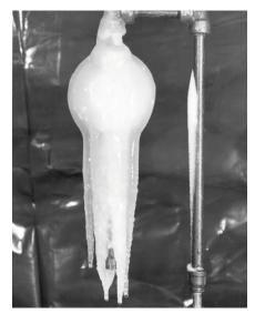
ICE COMPLETELY COVERED THE REGULATOR FISHER™ CONTROLS USED IN THE FREEZE TESTS.
