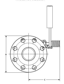
TYPE N551-24F WITH LATCH BLOCK OR TYPE P327D PNEUMATIC RELEASE
