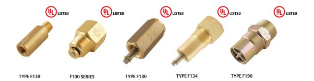
Excess flow check valves are intended to close upon excessive discharge of vapor or liquid resulting from a break in the hose or piping system. They are used to protect cylinder, tank and piping systems and are available in a large variety of sizes and body configurations. Standard temperature rating is -20 to  $160^{\circ}F$  / -29 to  $71^{\circ}C$ .
