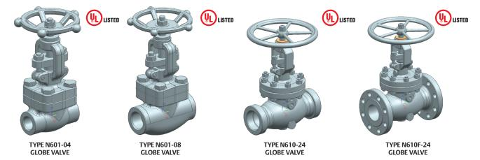
Globe and angle valves are widely used at bulk plants to control gas flow in the piping system, at storage tanks, on trucks and at pumps or compressors. Their body configuration permits installation in a straight section of pipe (globe body) or where it is desired to make a change in piping direction (angle body).
