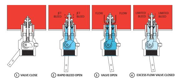
OPERATIONAL SCHEMATIC OF A TYPICAL FISHER INTERNAL VALVE
