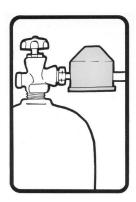
On single cylinder or domestic tank installations, it is frequently impossible to point the regulator's vent vertically down. Here an encasement or hood will be needed to protect the vent from the elements. Be sure the tank hood completely covers the vent.
