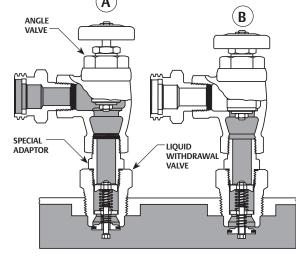
OPERATIONAL DRAWING OF A LIQUID WITHDRAWAL
