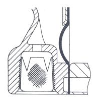
DRIP LIP VENT CONSTRUCTION HAS A RECESSED VENT OPENING WHILE THE NON-DRIP LIP VERSION ON THE RIGHT DOES NOT.
