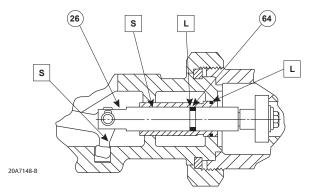
☐ APPLY SEALANT (S) / LUBRICANT (L)
