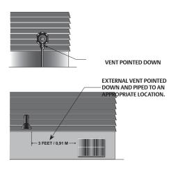
TYPICAL OUTDOOR INSTALLATIONS WITH REGULATOR VENT AND EXTERNAL VENT POINTING DOWNWARD
