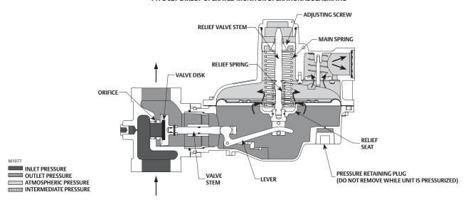
TYPE CS400IR INTERNALLY REGISTERED REGULATOR WITH INTERNAL RELIEF OPERATIONAL SCHEMATIC
