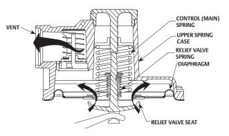
INTERNAL RELIEF VALVE BEING OPENED BY EXCESSIVE GAS PRESSURE
