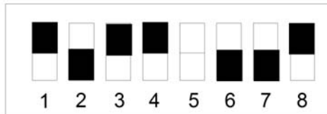
Figure 4.14 Type 1 DIP Switch Marked "OPEN" on Top of Switch, Default Settings.
