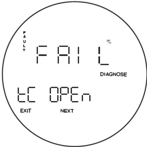
Figure 5-5. Fault 1, Open Thermocouple
