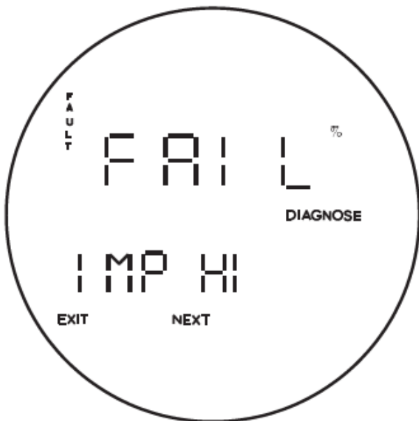
Figure 5-10. Fault 6, Cell Impedance Too High
