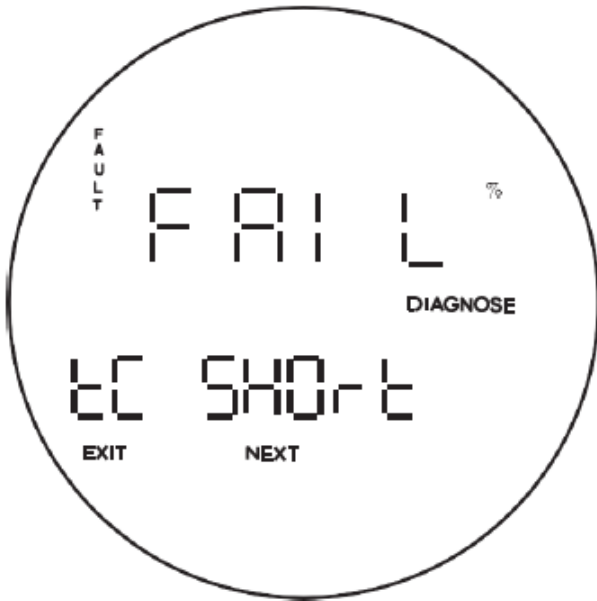
Figure 5-7. Fault 3, Shorted Thermocouple
