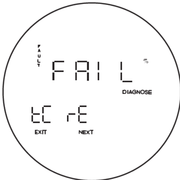
Figure 5-6. Fault 2, Reversed Thermocouple
