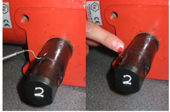
Step 8) Tap shaft inward to expose second seal groove. Install seal as per step 6.
