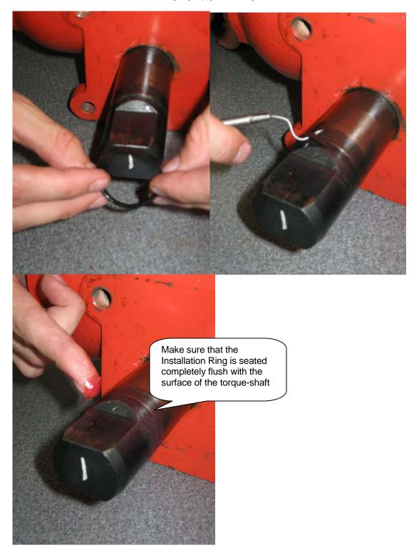
Step 5) Place Installation Ring into Rotor Clip groove of side 1. Use a pick or similar tool to aid installation. When shaft is fitted with ring, lightly grease ring surface.
