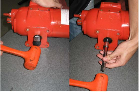
Step 3) Use the Pick to remove old seal and clear groove of old grease and debris.
