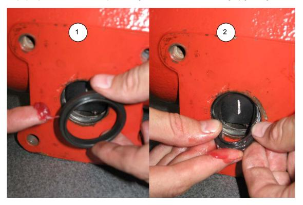
When installing, insert the top of the seal first, with the lip side inward towards shaft, then work the sides in. When the seal is mostly in, invert the bottom of the seal (see photo #3) into a wave like shape. When you release, the seal should seat itself smoothly into the groove. Press the seal in from all angles with your finger to make sure it is flush with the housing bore (see photo #4).
