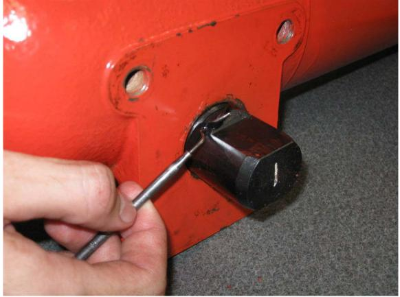
Step 11) On side 1, place Rotor Clip on torque-shaft. Tap this side towards the housing, pressing the Rotor Clip against the housing This makes it easier to remove the side 2 Installation Ring.
