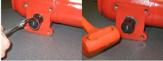
Step 12) Remove and discard side 2 Installation Seal and then install a new Rotor Clip
