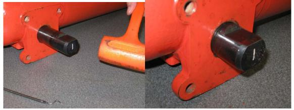
Step 10) Remove side 1 Installation Ring and discard.
