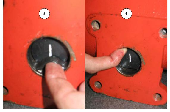
Step 7) On side 2, place Installation Rings on torque-shaft. Lightly grease as per step 5.
