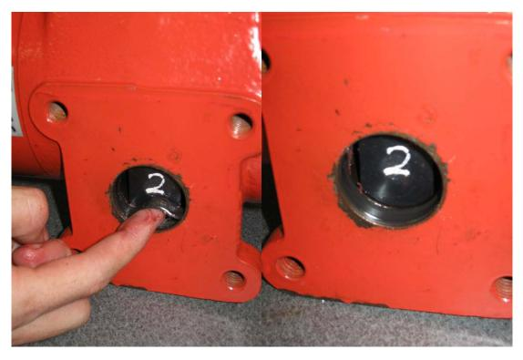
Step 9) Carefully tap torque-shaft back through housing and newly installed seals. If resistance is felt (a bouncy feeling especially), gently tap forward and backward until it becomes easier.
