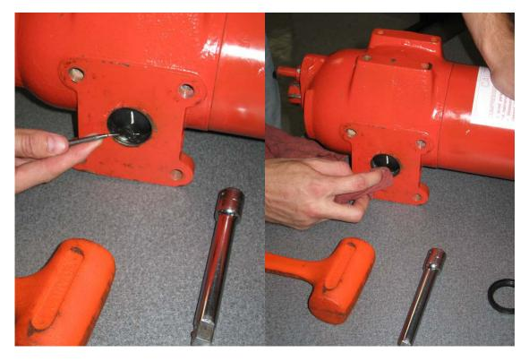
Step 4) Turn actuator to second side (side 2) and use Rotor Clip Pliers to remove rotor clip, tap shaft to expose seal, remove old seal and clean groove by repeating steps 1-3.
