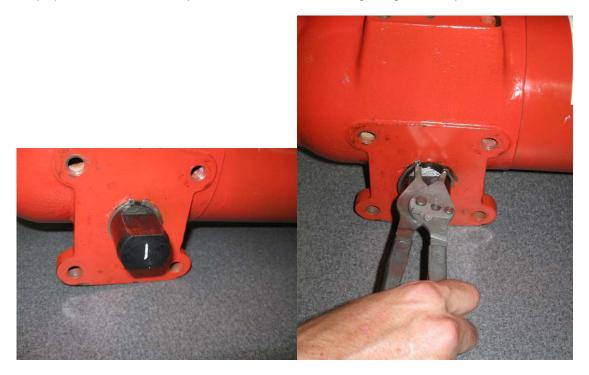
Step 2) Use the mallet to tap the torque-shaft inward with the use of an extension rod to expose the existing seal.
