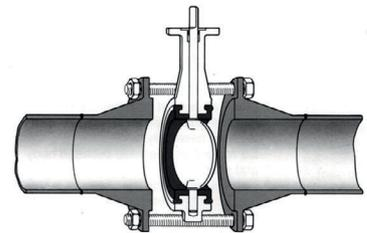
1. Spread the flanges with the adequate tooling. Insert some flange bolts to bear the valve
