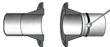
3. Remove the valve and finish weld. Install the valve according to the procedure in the left column.
