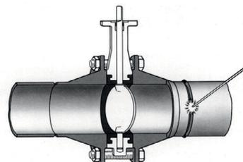
2. Tack weld the flanges to the pipes.
