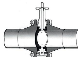
3. Close the valve clockwise, return to open position and cross-tighten all bolting.
