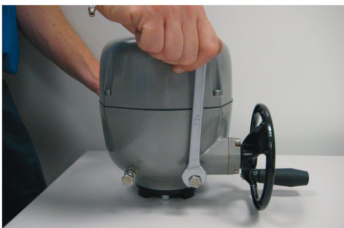
Figure 8 Setting of the Mechanical Stop
