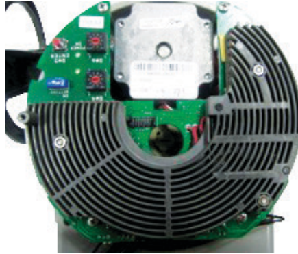
Figure 5 Example of EPI2 old version (heatsink present)
