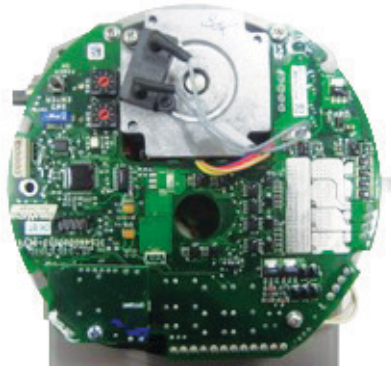
Figure 6 Example of EPI2 old version (heatsink not present)
