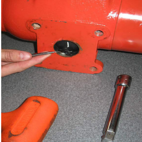
Figure 4 Cleaning the groove - Side 1
