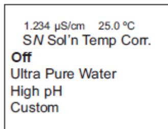
Figure 7-5: Solution Temperature Correction Screen
