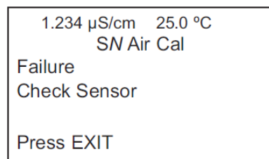
Figure 8-33: Air Cal Failure
