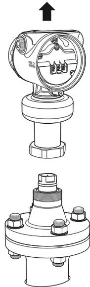
8. Attach a protection plug to the process seal to protect it from dust and water.
