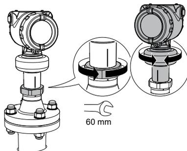
2. Verify the transmitter head is properly aligned.
