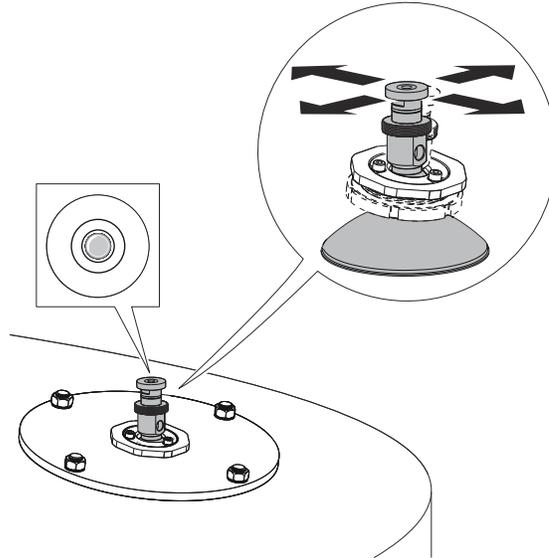
5. Gradually tighten the M8 screws.
