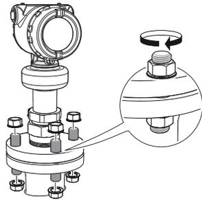
8. Screw the adapter until it is properly tightened.
