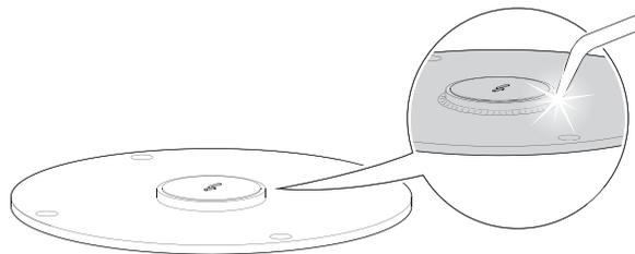
3. Remove the protection plates and visually inspect the internal surfaces of the flange ball for damage and dirt.
