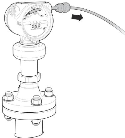
6. Loosen the nut that connects the transmitter head to the process seal.
