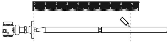
4. Remove and cut the segment at the marking.
