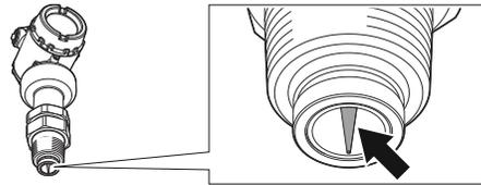
4. Screw the transmitter into the holder.
