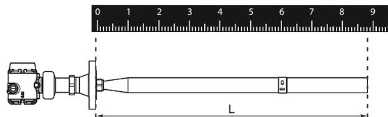
9. Update the transmitter configuration to the new Antenna Extension Length (L).
