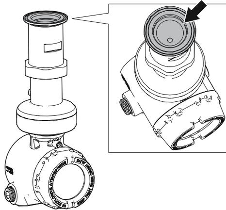
2. Verify the O-ring on the PTFE sealing is in place.
