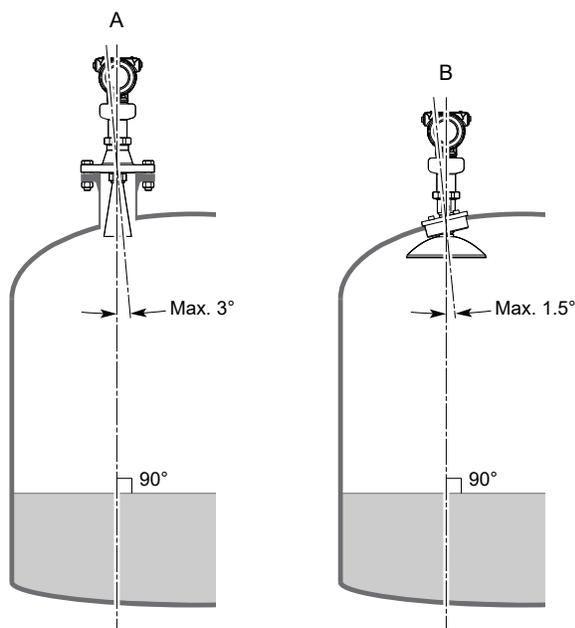
A. Cone antenna/process seal antenna
