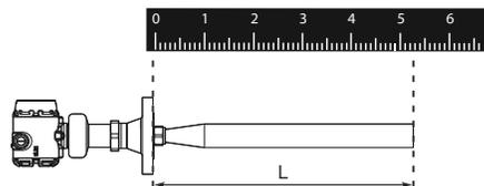
6. Update the transmitter configuration to the new Antenna Extension Length (L).
