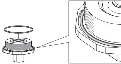
3. Mount the antenna adapter on flange/manhole cover. Ensure the antenna adapter fits tightly to the flange/manhole cover.
