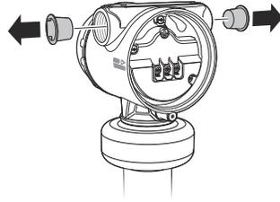
4. Pull the cable through the cable gland/conduit.<sup>(2)</sup>
