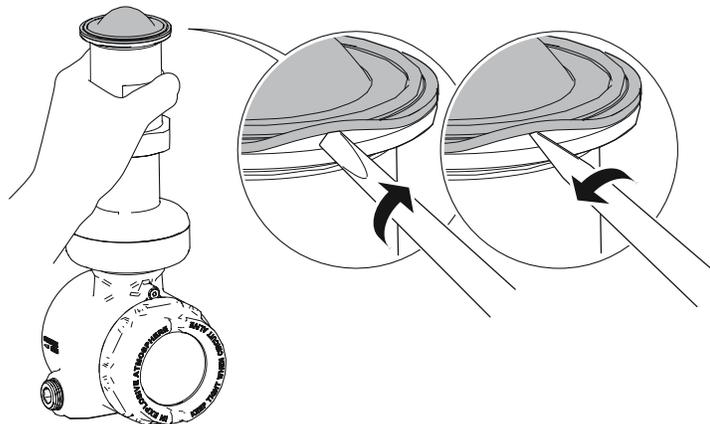
3. Repeat [Step 1-Step 2](#) at different positions until the PTFE sealing is loose.
