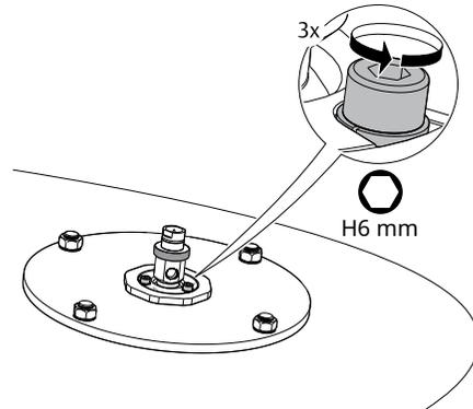
2. Rotate the antenna so the air purge connection is directed toward the tank wall.
