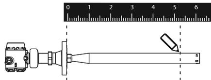
3. Cut the antenna at the marking.
