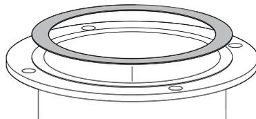
2. Lower the flange and antenna assembly into the nozzle.
