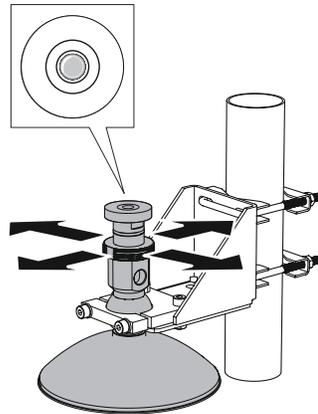
5. Gradually tighten the two M8 screws.
