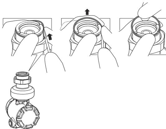
2. Replace the transmitter head nut.
