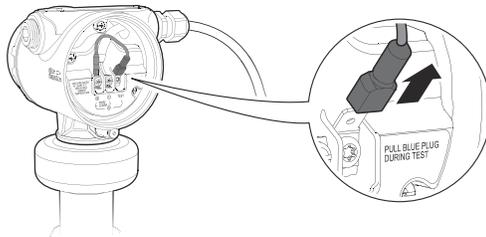
4. Connect the ampere meter leads to the terminals labeled "+" and "TEST".
