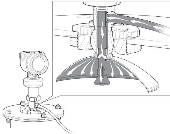
An air purge connection is also available for cone antennas with flanged connection by selecting option code PC1. This option consists of an antenna with purge holes and a separate air purge ring (see [Figure A-11](#)).
