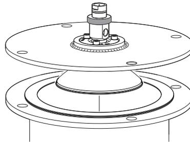
12. Tighten the bolts and nuts with sufficient torque for the flange and gasket choice.
