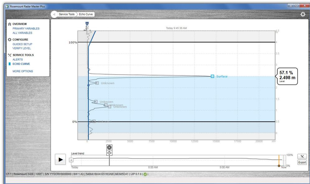
When connected to Rosemount Radar Master Plus, past measurement records and echo curves including the 10 highest peaks, as well as the 50 last alert events are automatically transferred from the transmitter's internal memory to the hard drive on your local computer. Past measurement records are then available the next time you connect to the transmitter using the level trend timeline.
