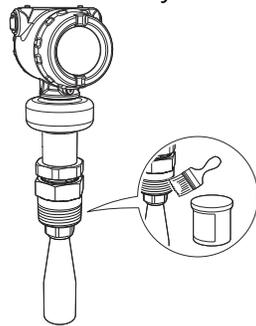
2. Mount the transmitter on the tank.
