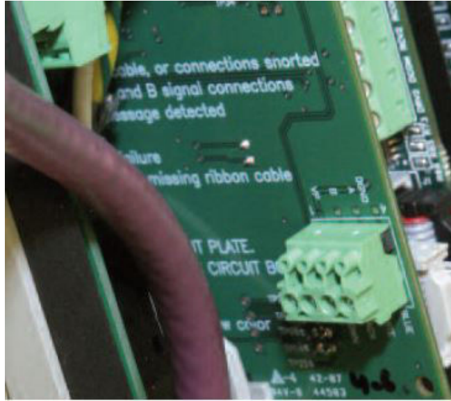
Figure 12-3: PROFIBUS Board Showing Removable 4-Lead Terminal Block
