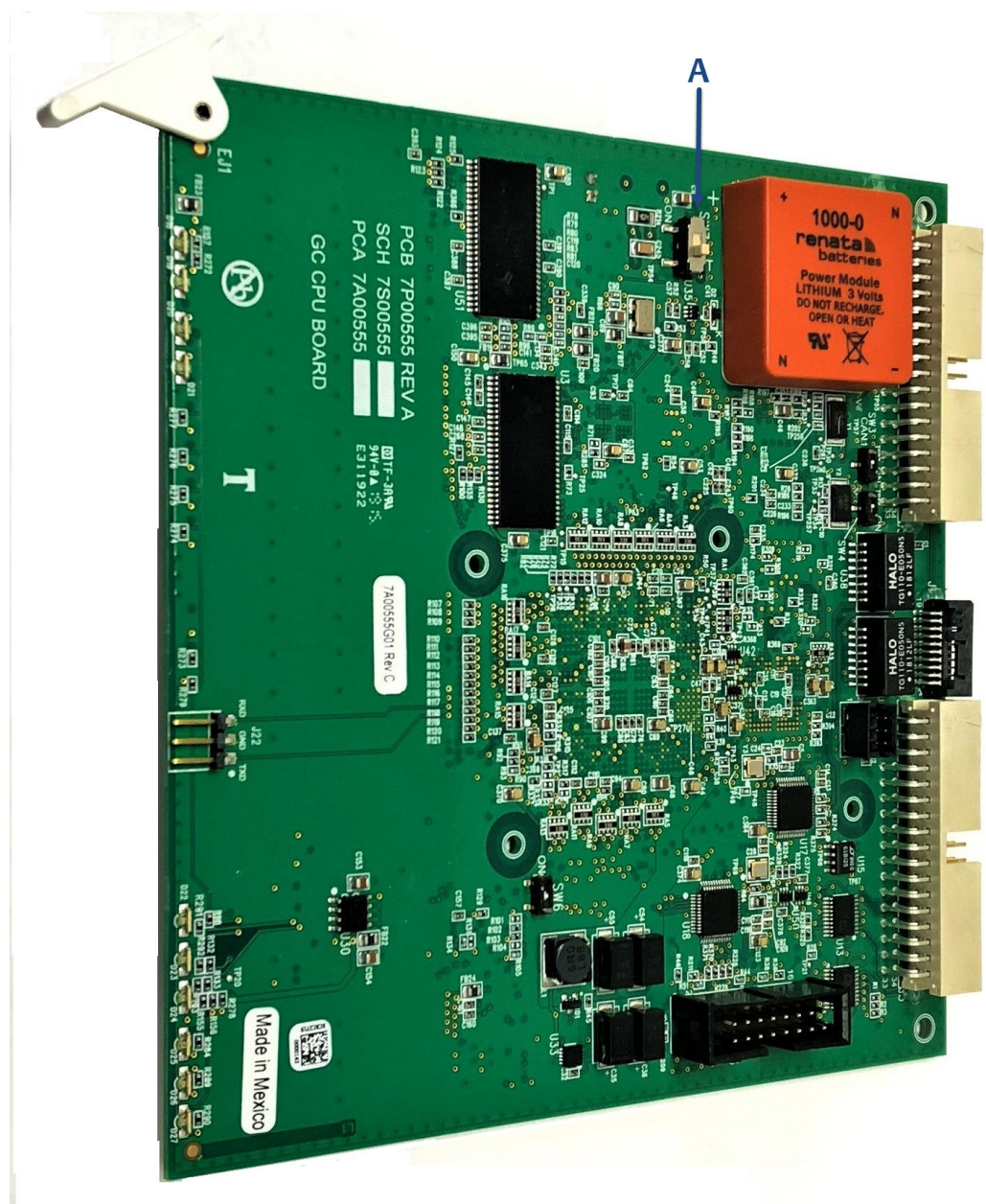
Figure 6-2: SW7 on the central processing unit (CPU) board
