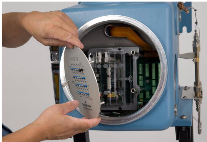
Figure 6-43: Remove the switch panel or LOI
