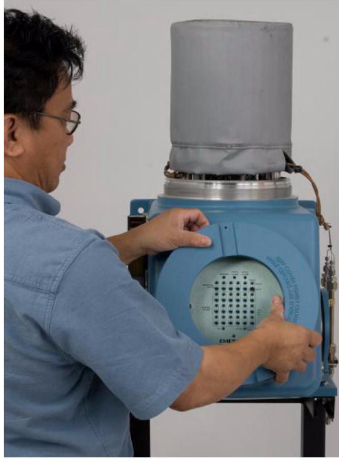
Figure 6-42: Remove the front panel
