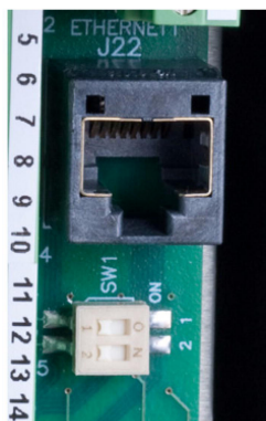
Figure 5-11: SW1 Switches on the Backplane
