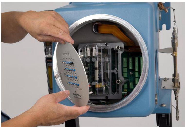
Figure 6-47: Removing the switch panel or LOI
