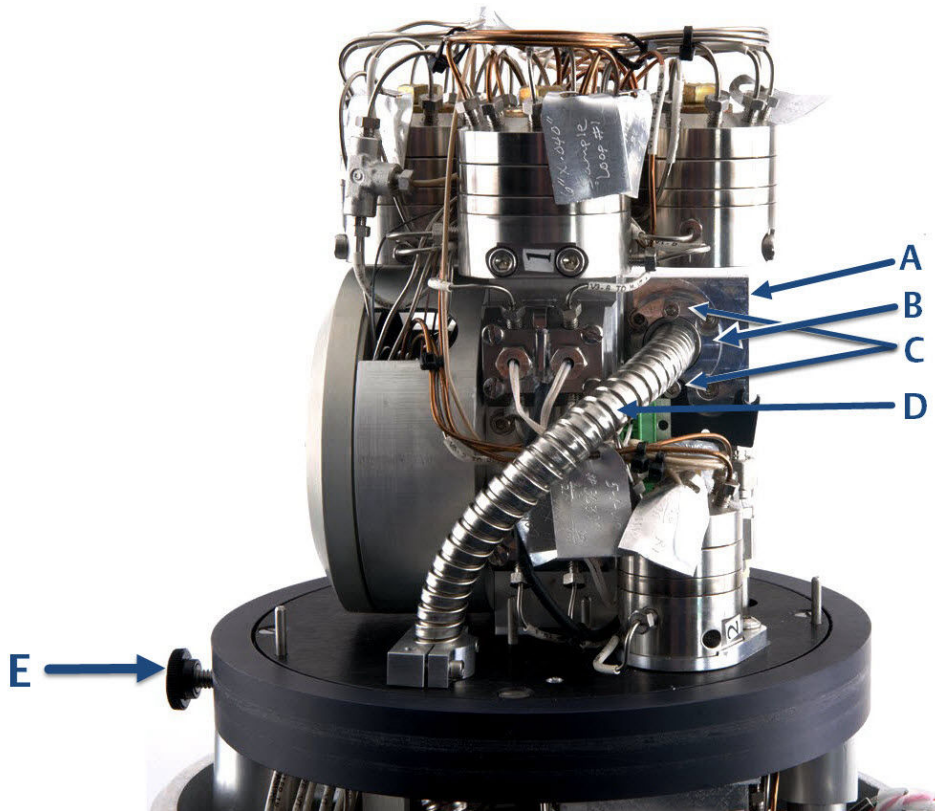
Figure 6-39: \mu FPD fiber cable assembly
