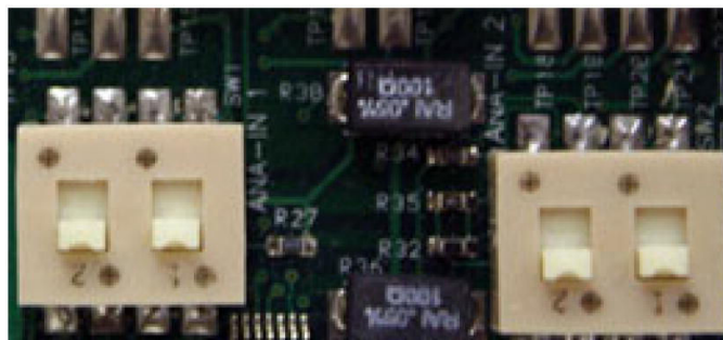
Figure 5-26: Factory Settings for Analog Input Switches
