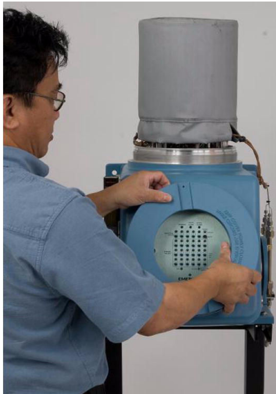
Figure 6-46: Removing the front panel
