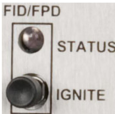
Figure 3-5: FID/FPD status LED
