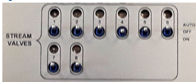
Figure 3-3: STREAM VALVES Switches
