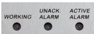
Figure 3-4: Status Light-Emitting Diodes (LEDs)
