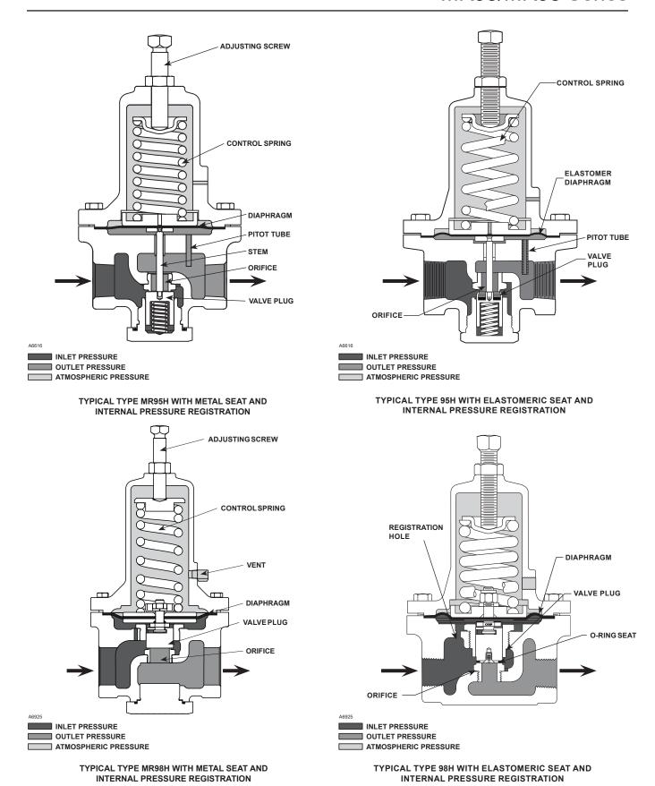
Figure 2. Typical MR95/MR98 and 95/98 Series Operational Schematics
