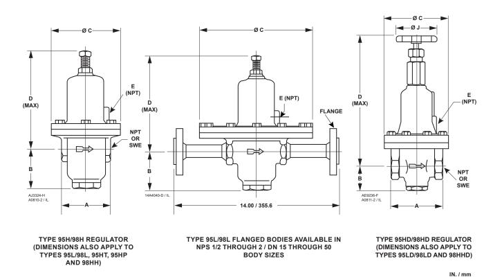
Figure 4. Typical 95 and 98 Series Dimensions
