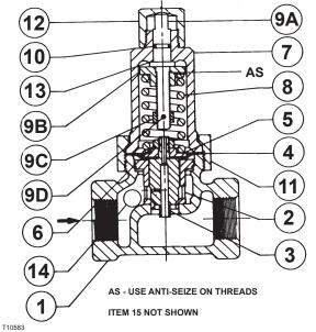
Figure 3. Type N110 Bypass Valve
