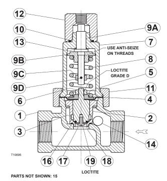
Figure 2. Type N120 Back Pressure Valve
