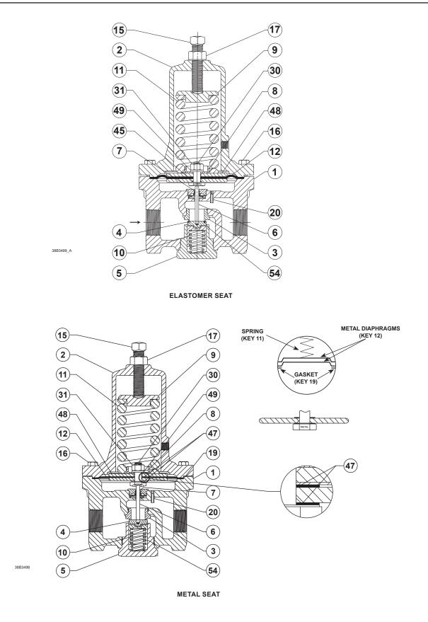
Figure 5. 95H Series, NPS 1-1/2 and 2 / DN 40 and 50 Sizes Assemblies (Also Typical of 95HT)
