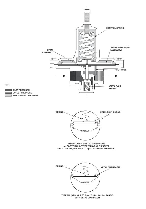
Figure 2. Type 95L with Metal Seat and Diaphragm Operational Schematic (Also Typical of Type 95H or 95HT)
