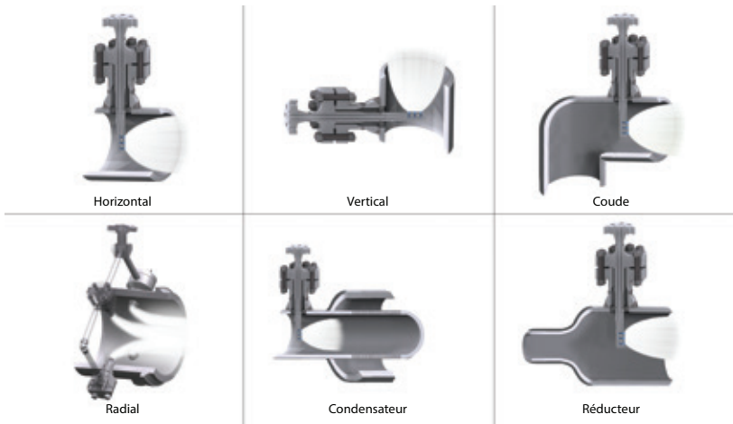
Figure 7.2 Installations de désurchauffage
