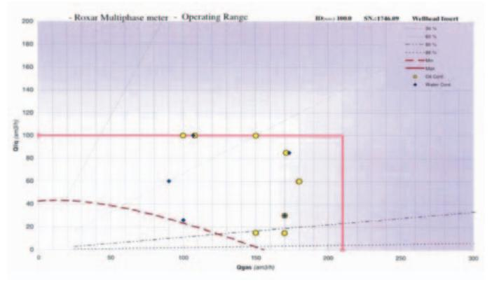
Figure 5. The operating range of the meter with CMR test points included.
