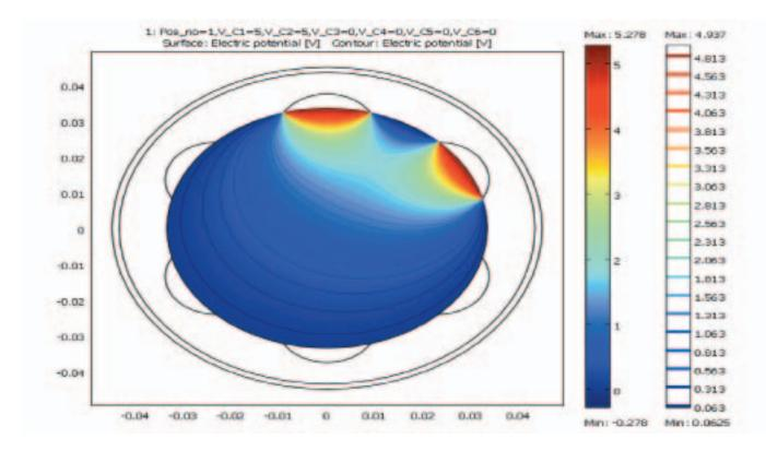
Figure 2. The new measurement principle behind the meter with red indicating high sensitivity and blue low sensitivity.
