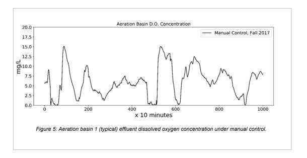
Automation of secondary controls was introduced in two phases with the goal of reducing variation and excess oxygen use. The first phase focused on automating aeration basin mixed-liquor depth control through influent-effluent flow balancing. The second phase automated aeration-based effluent D.O. concentration control through model predictive control (MPC).
