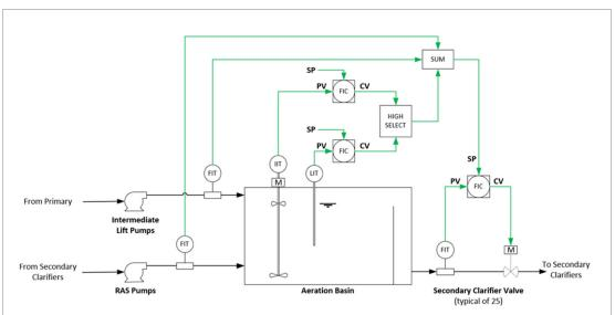
Figure 6: Depiction of the level control logic. Flow (FIT), mixer current (IIT), and level (LIT) transmitters are indicated. The three flow controllers (FIC) are depicted with setpoint (SP), process variable (PV) and controlled variable (CV) labelled. (Details in text).
