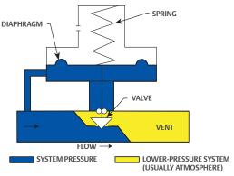
Figure 3. Direct-Operated Relief Valve
