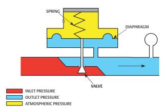
Figure 1. Direct-Operated Regulator
