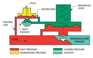
Figure 4. Pilot-Operated Relief Valve
