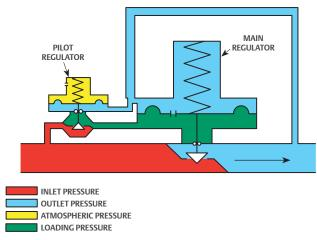
Figure 2. Pilot-Operated Regulator
