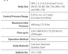
The Type 1190 provides very accurate pressure control on low-pressure blanketing systems. The regulator helps to control emissions and provides protection against any contamination from atmospheric conditions.
