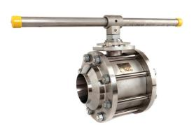
3-piece ball valves with ISO top flange DN 65 - DN 250 Butt weld, threaded, socket weld and flanged version.
