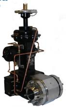
V300 Vee-Ball valves have a shearing action between the V-notch ball and the ball seal promotes a smooth, non-clogging operation. Unrestricted straight-through flow design provides high capacity for gas, steam, liquids.
