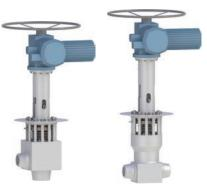
Electric-motor operated Gate and Globe valves for severe accident mode, capable to open at parameters up to 600 °C with a deltaP of up to 190 bars and able to stay open with pressurizer gas temperature up to 1200 °C. In addition, the valves are operable in the feed and bleed conditions.
