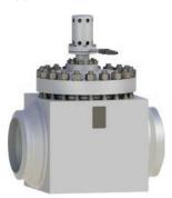
A swing check valve suitable for steam and water with a one-piece block-design. A special retaining ring assembly enables precise flap positioning. The lack of a shaft duct excludes leakages to the outside and ensures the function is not impaired by friction in the glands.
