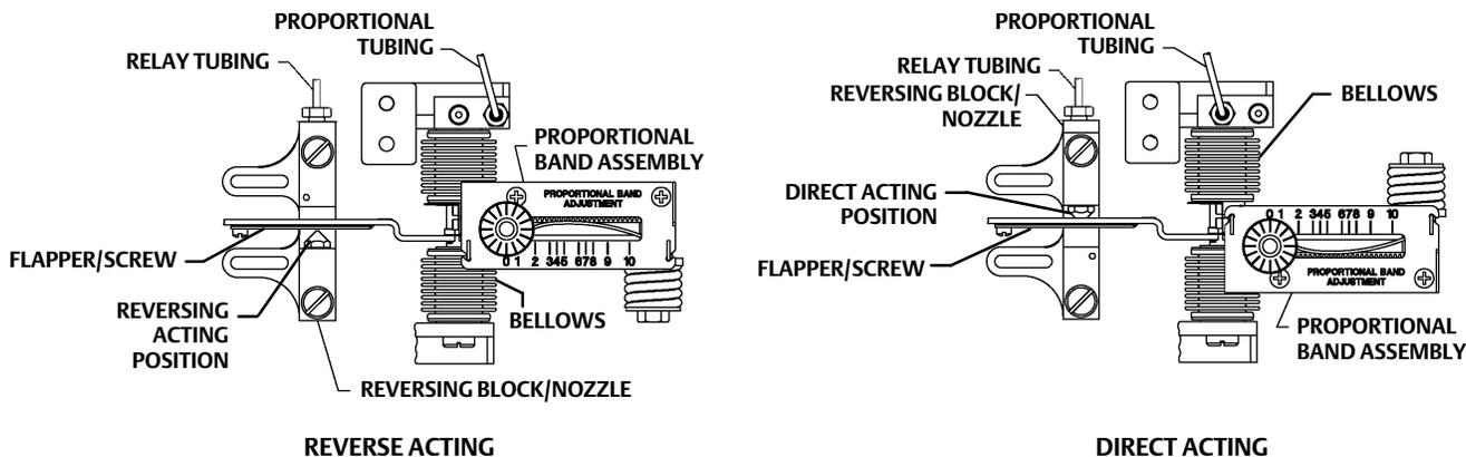
TO CHANGE ACTION OF THE CONTROLLER, REPOSITION THE PROPORTIONAL TUBING, REVERSING BLOCK/NOZZLE AND PROPORTIONAL BAND ASSEMBLY AS SHOWN ABOVE
