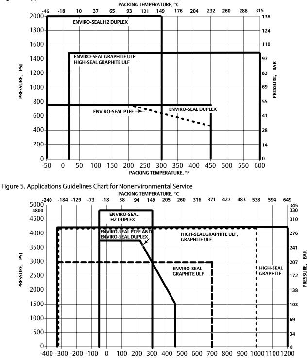
Figure 4. Applications Guidelines Chart for 100 PPM Service
