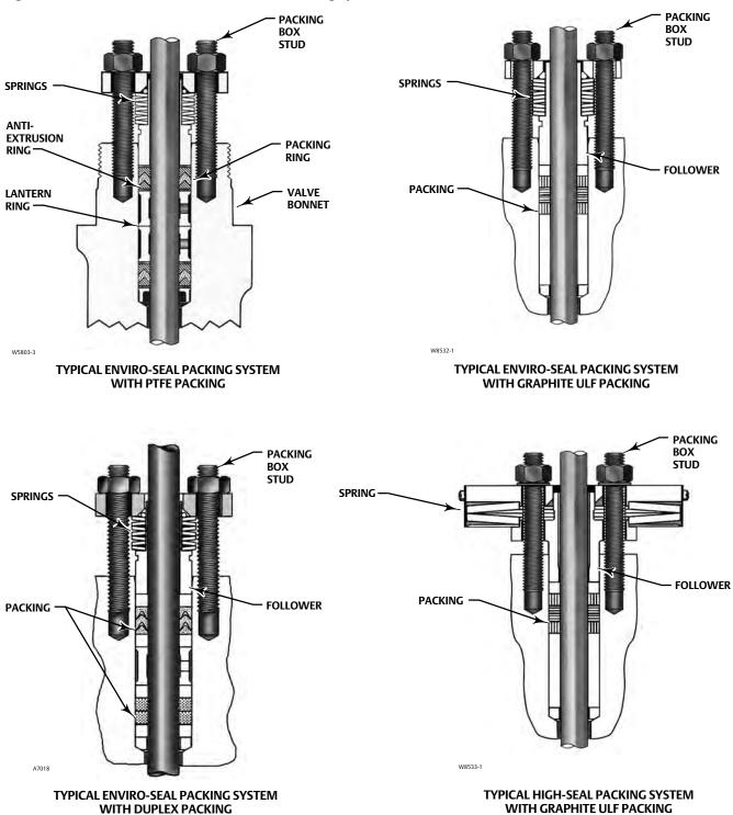
Figure 1. Fisher ENVIRO-SEAL and HIGH-SEAL Packing Systems
