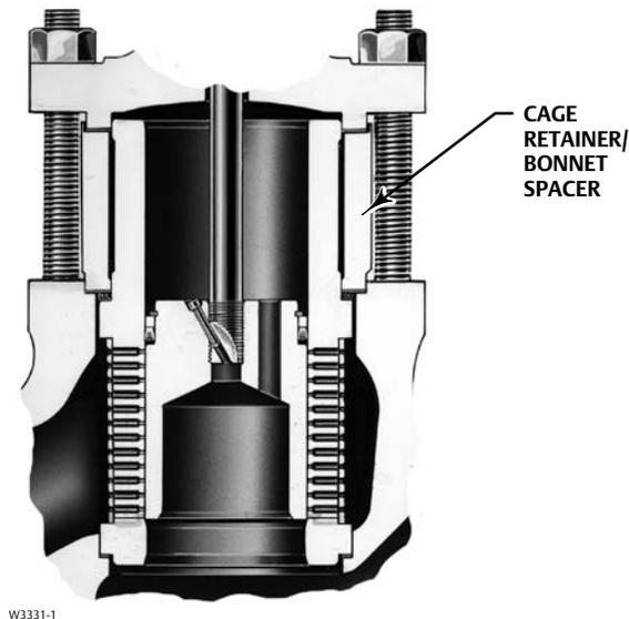
Figure 12. Typical Trim Used in Cavitrol III Cage Constructions with Steel or Stainless Steel Valves (see tables 15)
