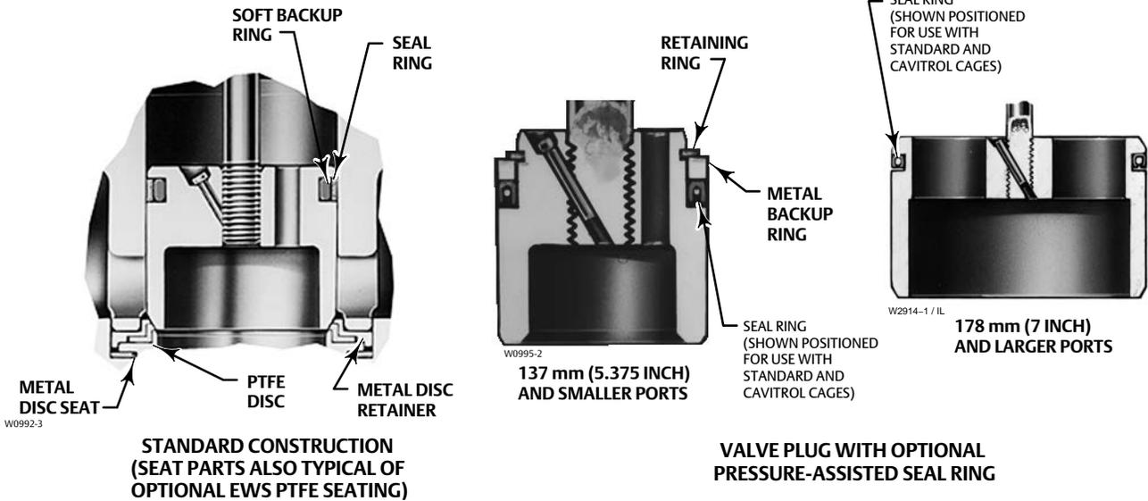
Figure 3. Fisher EWS Trim Details Showing Standard Cage and Seating Construction
