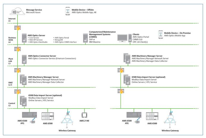
The AMS Machinery Manager Data Collector allows for flexible, yet secure, installation. Once installed you can monitor your system within minutes.
