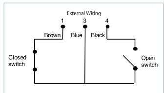
Switches shown in closed valve position. Max. cont. load 2.5 W. Insulation tested to 1000 V.
