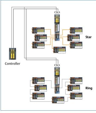
Distributed CHARMs architecure with DeltaV SIS with Electronic Marshalling.
