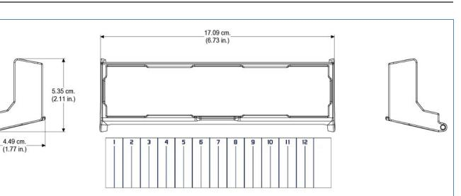
Horizontal Channel Identifier Label/Wiring Cover for CHARM I/O Block.
