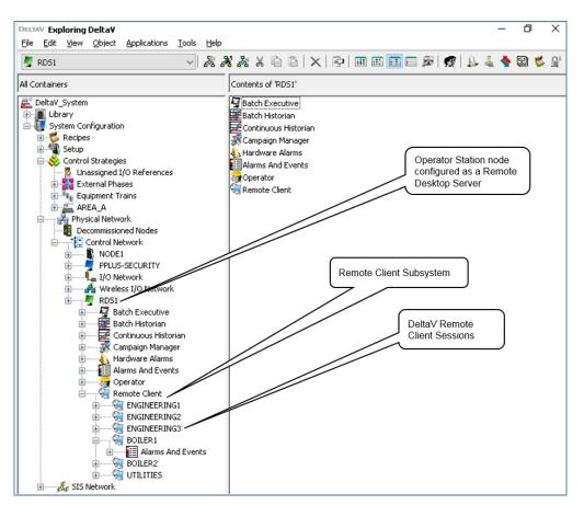
DeltaV Explorer showing setup for Remote Clients.
