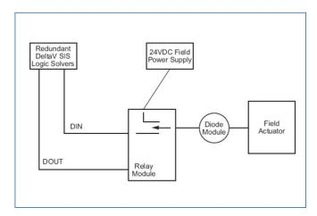
Relay module block diagram.
