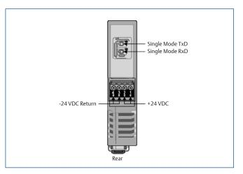
Single Mode Fiber-Optic Connectors on the SISNet Distance Extender (Top View).
