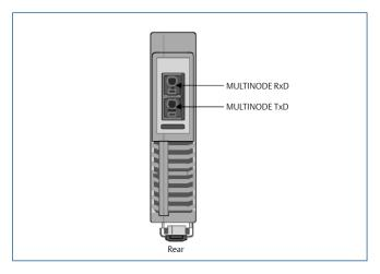
Multimode Fiber-Optic Connectors on the SISNet Distance Extender (Bottom View).
