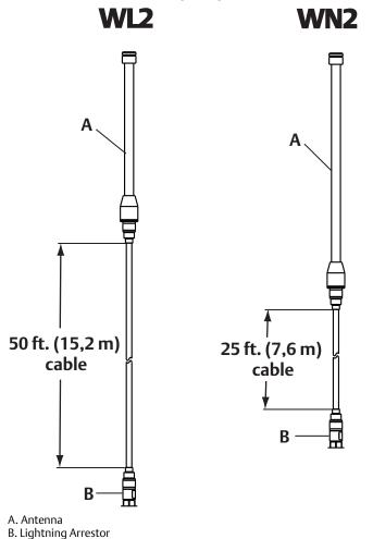
Figure 4. SMA to N-Type Adapter Cable Dimensions
