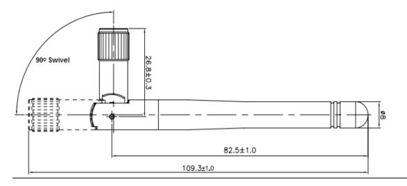
Figure 3. Remote Omni-Antenna Kit
