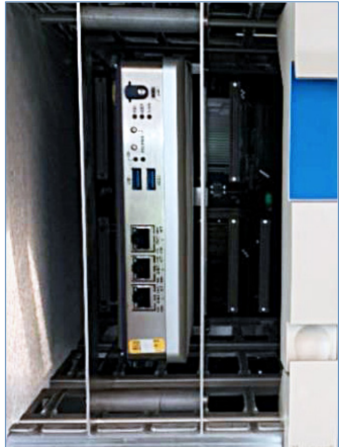
Figure 4. Vertical Mounting in I/O File.
