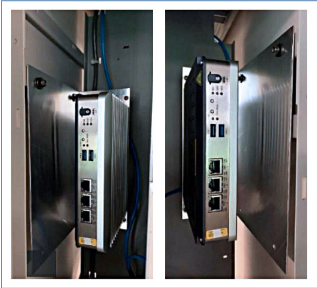
Figure 5. Vertical Mounting on Rails, Left & Right Sided.
