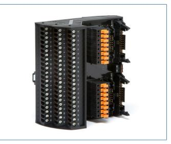
The AI/AO Plus Mass Connection Board connects to the **M-series Plus** (simplex or redundant) **AI**, **16 Channel and AO**, **16 Channel** cards by using either two ribbon cables with 24-pin connectors or the 48-pin special Round Ribbon Cable, which is required if the distance is longer than 3m.
