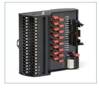
The DI Plus Mass Connection Solution (set of two boards) connects to the **simplex or redundant M-series Plus DI**, **32 Channel, 24V DC, Dry Contact cards** by using either two ribbon cables with 20-pin connectors or two of the 20-pin standard Round Ribbon Cable, which is required if the distance is longer than 3m.
