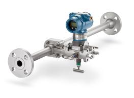
Rosemount 3051CFP Integral Orifice Flow Meters enable highly accurate flow measurement in small line sizes. Internal pipe diameter variation in combination with plate centering issues can greatly magnify flow measurement errors in small line sizes. Integral Orifice Flow Meters use a precision honed pipe section to minimize internal pipe diameter variation along with a selfcentering plate design to eliminate alignment errors.
