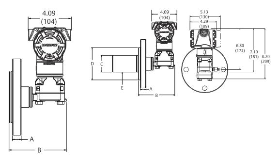
E. 2-, 4-, or 6-in. extension (only available with 3- and 4-in., DN80, and DN100 flange configurations)
