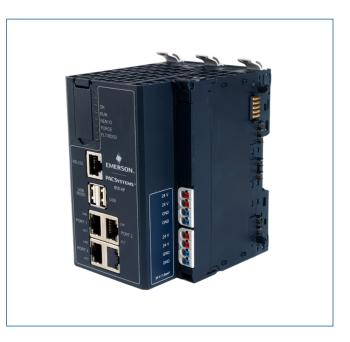
The RSTi-EP CPE200 compact controller series is designed to enable supply chain flexibility. We have built-in open communications to allow you to easily connect a very wide range of 3rd party devices. With real time I/O networking capabilities, up to 3x 1-Gbps Ethernet ports and support of all popular communication protocols including PROFINET<sup>©</sup>, OPC UA, Modbus/TCP, and DNP3 the RSTi-EP CPE200 compact controller gives you the resilience to succeed.
