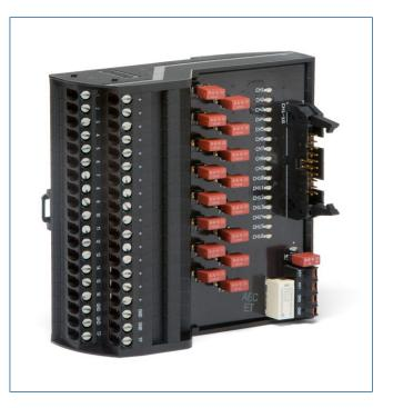
This DI Mass Connection Solution (set of two boards) connects to the **existing simplex S-series DI, 32 Channel, 24 VDC, Dry Contact cards** by using either two ribbon cables with 20-Pin connectors or two of the 20-Pin standard Round Ribbon Cable, which is required if the distance is longer than 3m.
