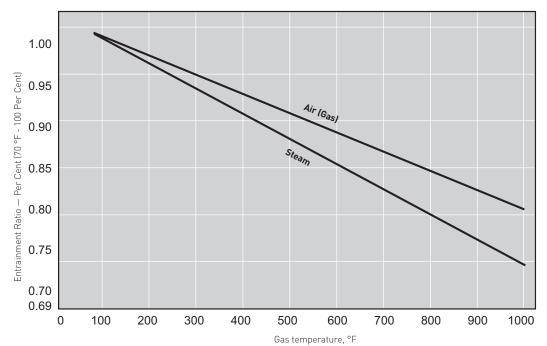
TEMPERATURE ENTRAINMENT RATIO CURVE (NO. 2)\*
