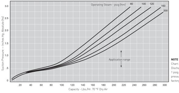
Chart is for maxium Discharge Pressure (hd) of 1 psig. If actual discharge pressure is greater, contact factory. L-4H PERFORMANCE CURVES
