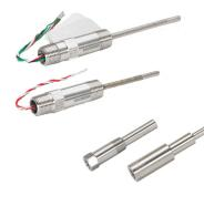
The 68 Series Sensors may be ordered as complete assemblies, by specifying type of sensing element, length, extension, and thermowell. They can be ordered with flying leads, or an enclosure (connection head) with terminal block.
