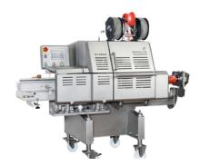
The SV4800 from Tipper Tie: The clip system for slicer ware and shaped products closes plastic, fiber, and collagen casing with diameters up to 160 mm at a rate of up to 120 cycles per minute.
