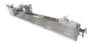
The automation design of the thermoforming machines enabled operators to switch over to different product sizes and types with one touch of a button.
