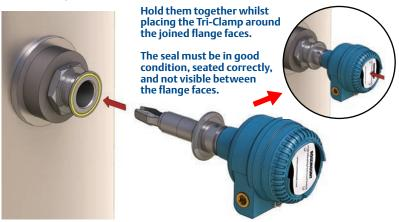
4. Place the Tri-Clamp around the joined flange faces and tighten the bolt(s).
