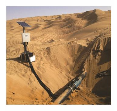
The Roxar FSM Log 48 Area Corrosion Monitor allows you to gain more control over the integrity of your pipeline, maximize transportation capacity and reduce operating expenses. The Roxar non-intrusive area monitoring technology provides unmatched capabilities for detecting general and localized internal corrosion.
