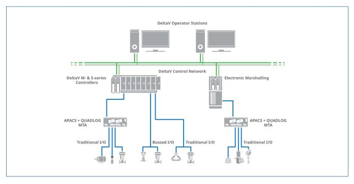
DeltaV\*\* Flex.Connect wiring solutions protect your wiring investment as you convert from APACS+ & QUADLOG to the DeltaV System.
