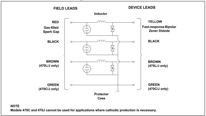
FIGURE 3. Schematic Diagram of Transient Protector Models 470D, C, L, and J.
