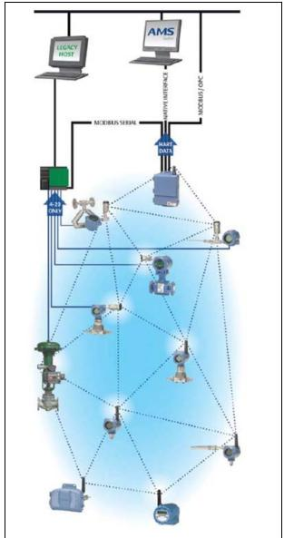
Smart Wireless Field Network containing wireless THUM Adapters and wireless instruments connected to any host system via the Smart Wireless Gateway.
