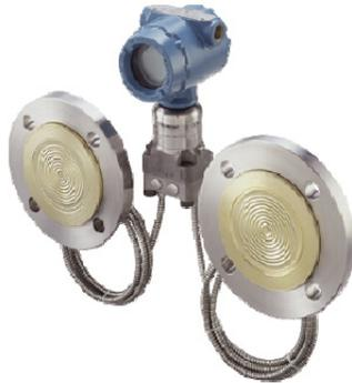
**Figure 1-4. A change in process temperature induces the fill-fluid density to change within the capillary. This change in density causes a measurement shift due to the head pressure varying.**
