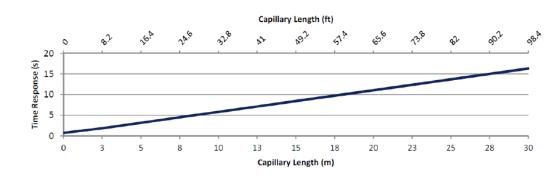
The time response of 1.092 mm (0.040-in.) capillary with Silicone 200 fill-fluid at 24  $^{\circ}$ C (75  $^{\circ}$ F) ambient. System is balanced with equal lengths of capillary on the low and high reference connection of the transmitter.
