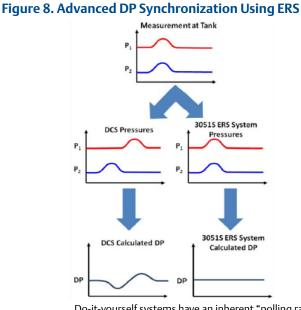
Do-it-yourself systems have an inherent "polling rate error" as the PHI and PLO signals are not synchronized.
