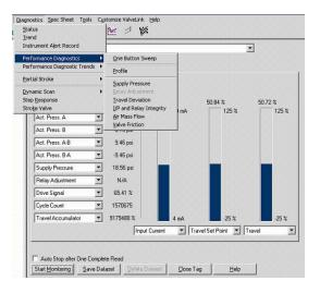
Common tests include a full signature test that checks valve response over the full valve stroke and measures seating pressure for full valve closure. These tests also monitor actuator pressure and valve movement. The One Button Sweep performs all these checks in a single diagnostic test.
