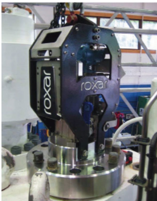
Figure 4. The fully installed meter.
